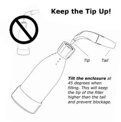
When using the filler, always **keep the tip of the filler higher than the tail** of the filler. Otherwise, the tip of the cartridge will be pointing downward, and liquid  $CO_2$  will flow into the regulator and block the flow of gas.
